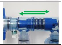
If the Venturi is not moving or moving intermittently and erratically, discontinue use 18. of the circuit and replace it with another circuit.
