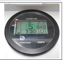
Ensure that the Pulse Frequency Rate is 500-600 Cycles Per Minute (CPM). Adjust if 16. needed using the **PULSE FREQUENCY** knob only.
